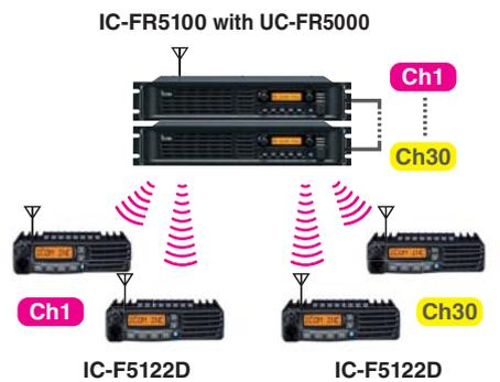
The IC-F5122D series can be used in an IDAS single-site trunking system. The IDAS trunking system is a distributed system with no dedicated control channel, so more voice traffic channels are available for increased system capacity.
