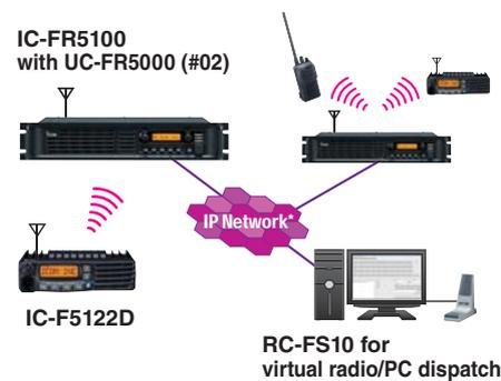
When using the IC-F5122D series in IDAS multi-site conventional mode, the IC-F5122D can communicate with other IDAS radio users working with other repeater sites and/or virtual radio/PC dispatch stations on the IDAS network.
