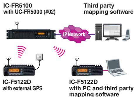
When used with an external GPS receiver, the IC-F5122D series can transmit accurate position data for use with vehicle management applications.
